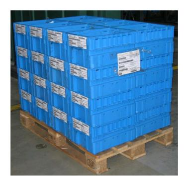
Adhesive stickers should not be attached when using VDA small load carriers.
